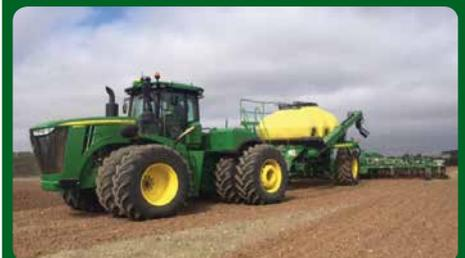
Seeding Demo at Booleroo Centre. John Deere 9420R pulling 1910 air cart and 40ft 1870 Conservapack with RTK guidance utilising ITEC Pro.
