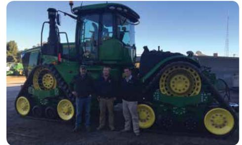
This John Deere 9520RX 4-Track machine, was the first one delivered in our group, running on 30" tracks, equip with John Deere RTK & a ProTrakker steering hitch. Pictured are customers Lyndon and Robert Price with Crystal Brook Sales Consultant Brock Scott.
