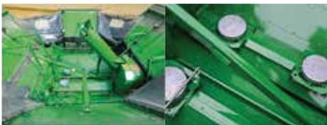
John Deere Active Yield (available on MY18 S700 series harvesters) can also be retrofitted to S600 series harvesters. These load cells mean no more weight yield calibrations to the chaser as the machine will do it for you!
